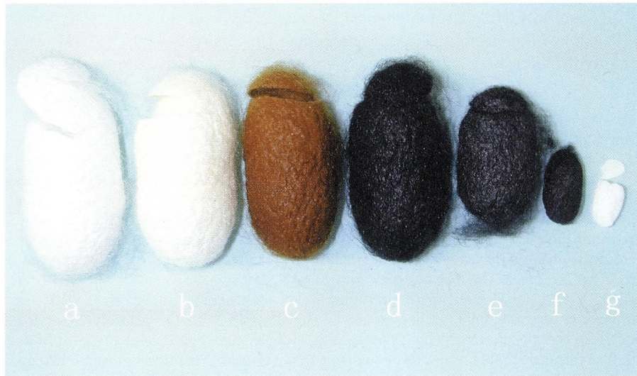
Figure 1 The B. mori cocoon shells subjected to increasing heat treatments.
