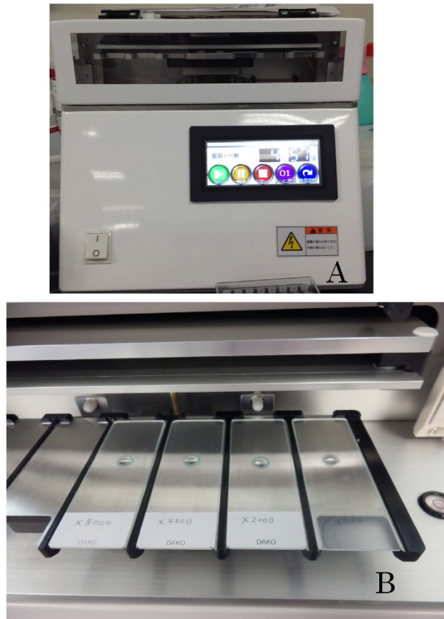
Figure 2. (A) The Histo-Tek® R-IHC®. (B) A 15- \mu l droplet containing antibody on the microscope slide between the electrodes.
