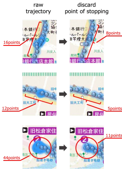
Figure 17. Examples of recognizing walking and stopping with the acceleration sensors' threshold value set at Th_2 = 0.1 G . Blue dots show every 15-second point of a user's trajectory data. Simplified trajectory data are effective in reviewing and playing back a user's trajectory on the screen.
