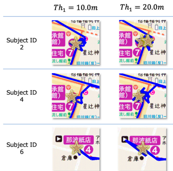
Figure 13. Results at which points of staying indoors were recognized with two different threshold settings, i.e., Th_1 = 10.0\text{ m} (left) and Th_1 = 20.0\text{ m} (right).
