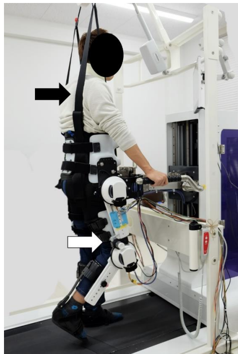
Figure 4. A walking training rehabilitation robot with functional electrical stimulation (FES) for paraplegia. The exoskeleton is made based on the long leg orthotic device, and the rehabilitation unloading lift (black thick arrow), FES and robot orthotic device (white thick arrow) are attached, and walking exercise is performed on the treadmill.
