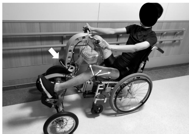
Figure 3. A new functional electrical stimulation (FES) cycling system. The FES cycling system consists of a front-wheel drive unit (thick white arrow) that can be attached to a standard wheelchair and an FES control part (thin white arrows) that enables cycling operation for lower limb paralysis.
