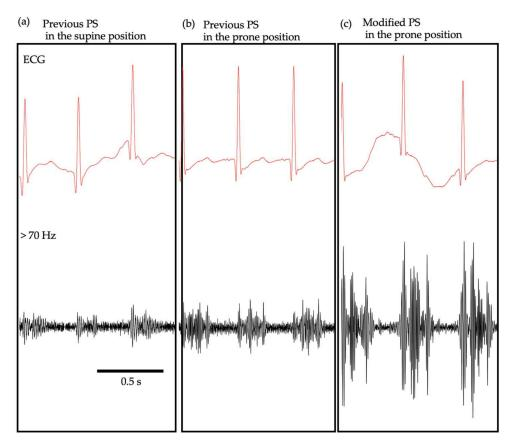
**Figure 2.** Comparison of heart sound signals and murmurs between the previous and modified PS. Simultaneous recording of ECG and the PS waveforms recorded with the previous PS in the supine (**a**) and prone (**b**) positions and the modified PS in the prone position (**c**). The PS waveforms were high-pass-filtered with a cut-off frequency of 70 Hz.
