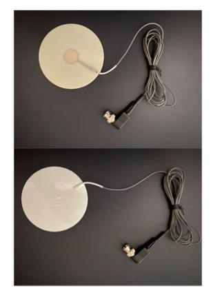
**Figure 1.** The appearance of the piezoelectric sensor (PS). The upper panel shows the bottom surface of the PS. The lower panel shows its top surface, which faces the patients. The diameter of the sensor is 100 mm. The sensor is covered with an insulation material.
