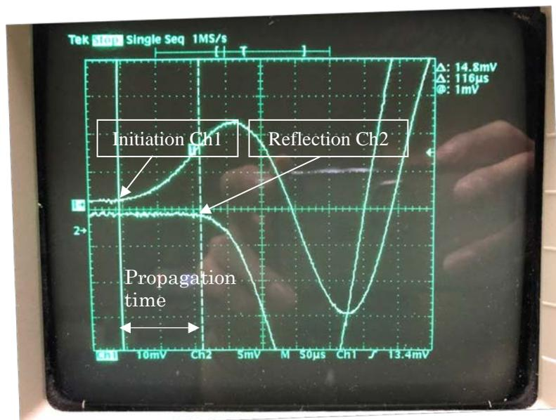
Figure 4. Example of elastic wave measurement in concrete pile Time  $50\mu\text{s}/\text{div}$ . Ch1  $10\text{mV}/\text{div}$ . Ch2  $5\text{mV}/\text{div}$ .
