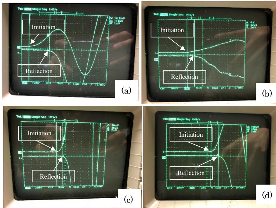
Figure 8 Elastic wave propagations of concrete on oscilloscope, (a) concrete pile having dimensions of 100×100×600 mm<sup>3</sup>, (b) concrete cube having dimensions of 200×200×200 mm<sup>3</sup>, (c) crashed concrete having no cracks, (d) crashed concrete with cracks. Time (a)~(d) 50μs/div. Ch1 (a), (b) 10mV/div. (c), (d) 20mV/div. Ch2 (a), (b) 5mV/div. (c), (d) 10mV/div.
