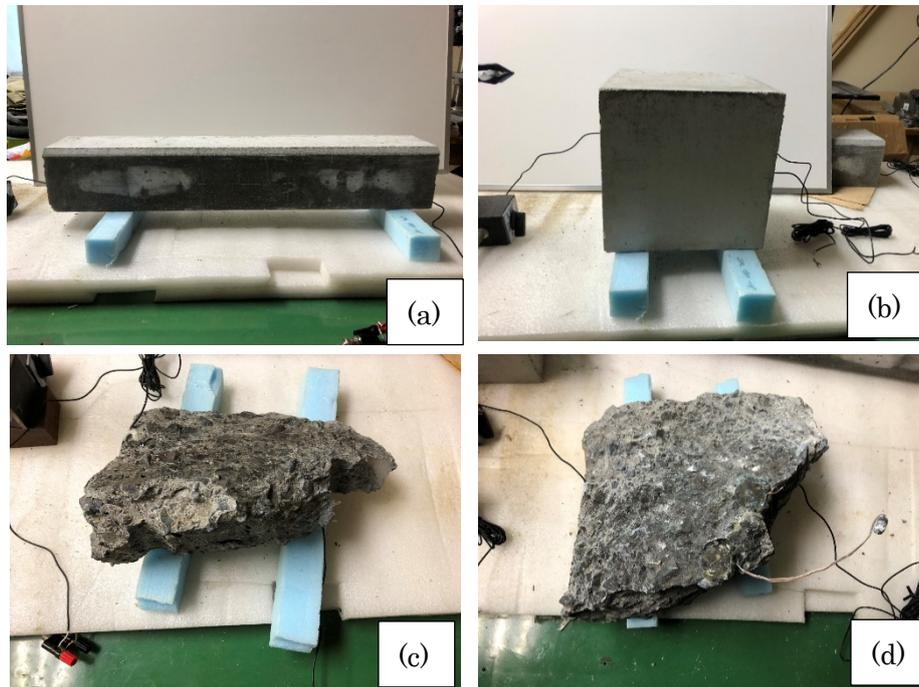
Figure 6. Concrete test pieces for EWV measurement, (a) pile of  $100 \times 100 \times 600 \text{ mm}^3$ , (b) cube of  $200 \times 200 \times 200 \text{ mm}^3$ , (c) crushed piece having approximately 400 mm length without cracks, (d) crushed piece having approximately 300 mm length with cracks.
