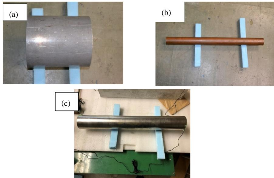
Figure 5. Setting of standard materials for EWW measurement, (a) Al, (b) Cu and (c) austenitic stainless steel (SUS304).
