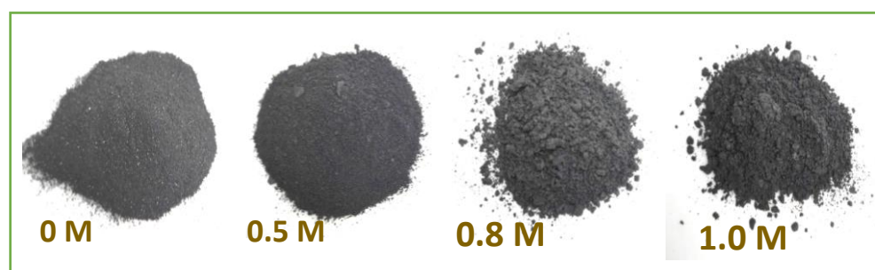
Figure 2.10: Residues obtained after atmospheric beaker leaching at different sulfuric acid concentrations.
