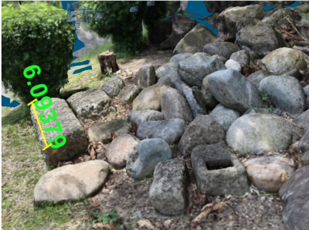
Figure 35. Close up of Set #2 meshed 3D CG reconstruction, with measurements on long rectangular prism-shaped rock that was used as reference.
