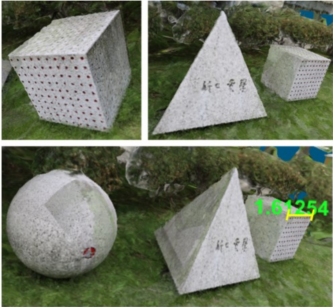
Figure 28. Mesh reconstructed 3D CG model of the monuments. 3 rd picture (bottom) shows measured side of cube monument when using 100 images.
