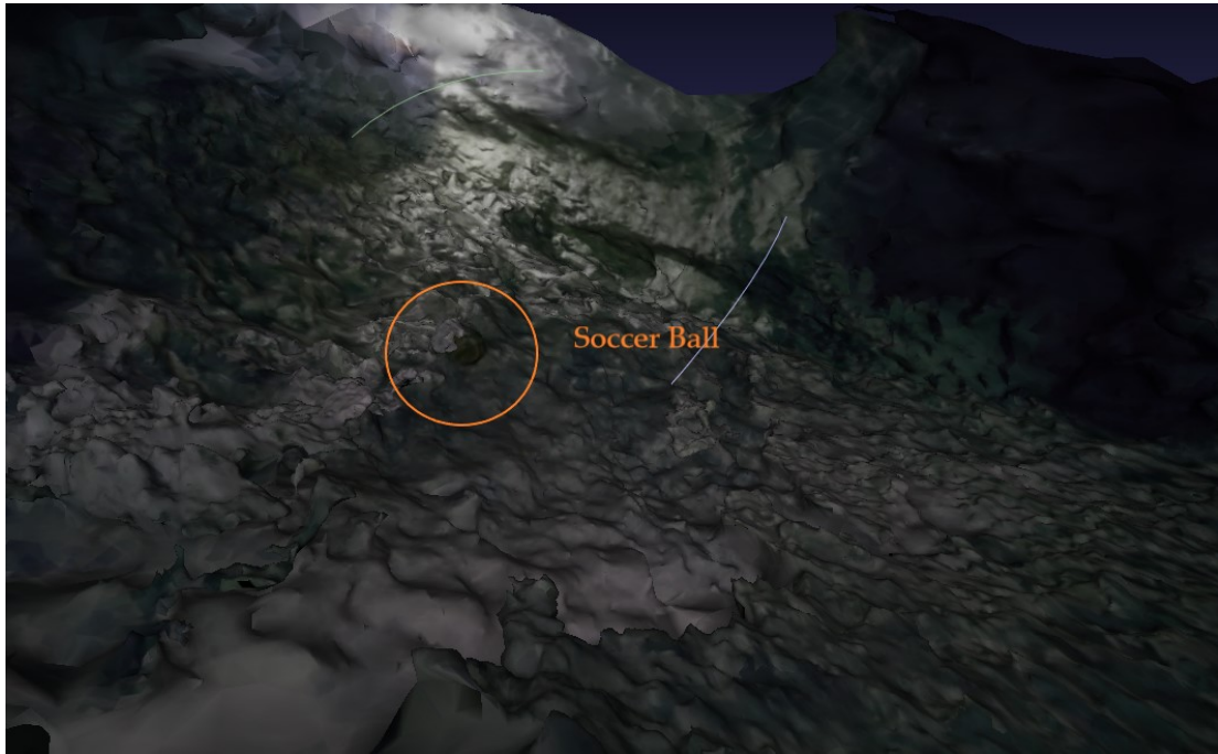
Figure 22. Close-up of the Textured Mesh generated by Meshroom. Note that the soccer ball is almost unidentifiable and the presence of floating 'blobs'
