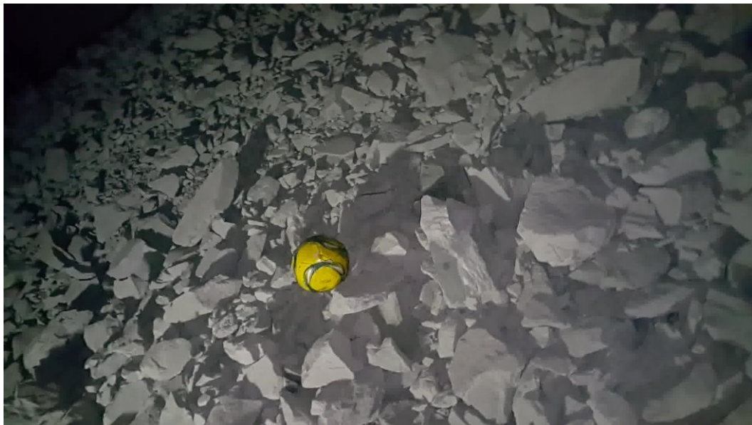
Figure 14. A single frame taken from the video of the muckpile. Presence of soccer ball for scaling purposes.
