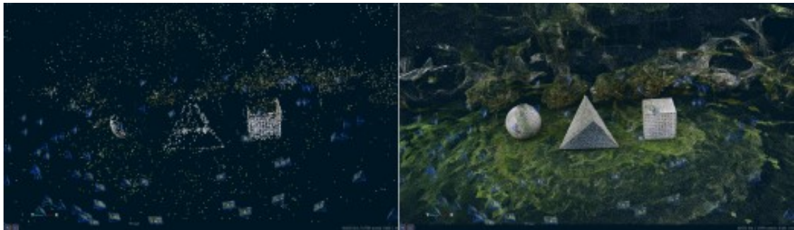
Figure 12. Sparse point cloud (Left) and dense point cloud (Right) of a scene.
