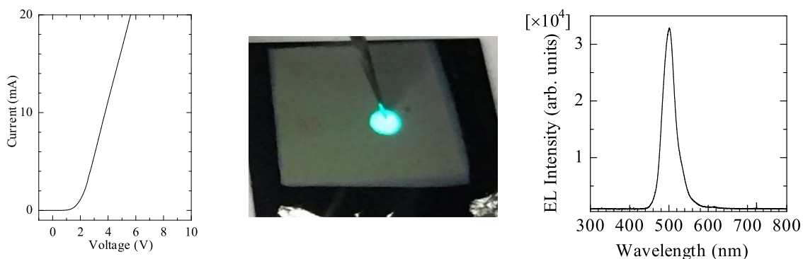
FIG. 2. I - V characteristic, photograph of light emission, and EL spectrum of the DH-type pn-junction diode directly grown on a mirror-polished multi-crystalline Si substrate.
