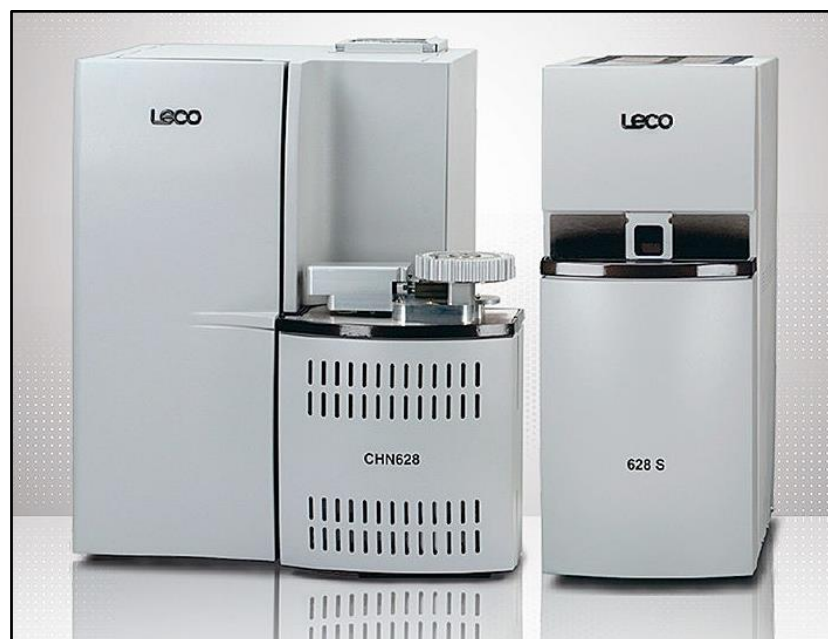
Figure 2.5. LECO CHNS628 elemental analyzer used in this study ( www.leco.com )
