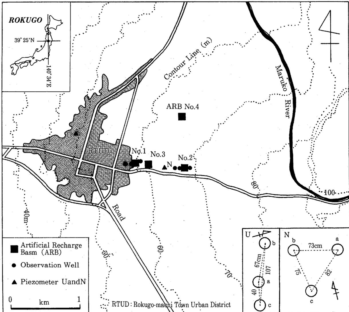
Figure 1. Nos. 1-4 artificial recharge basins for the unconfined aquifer in the Rokugo alluvial fan
