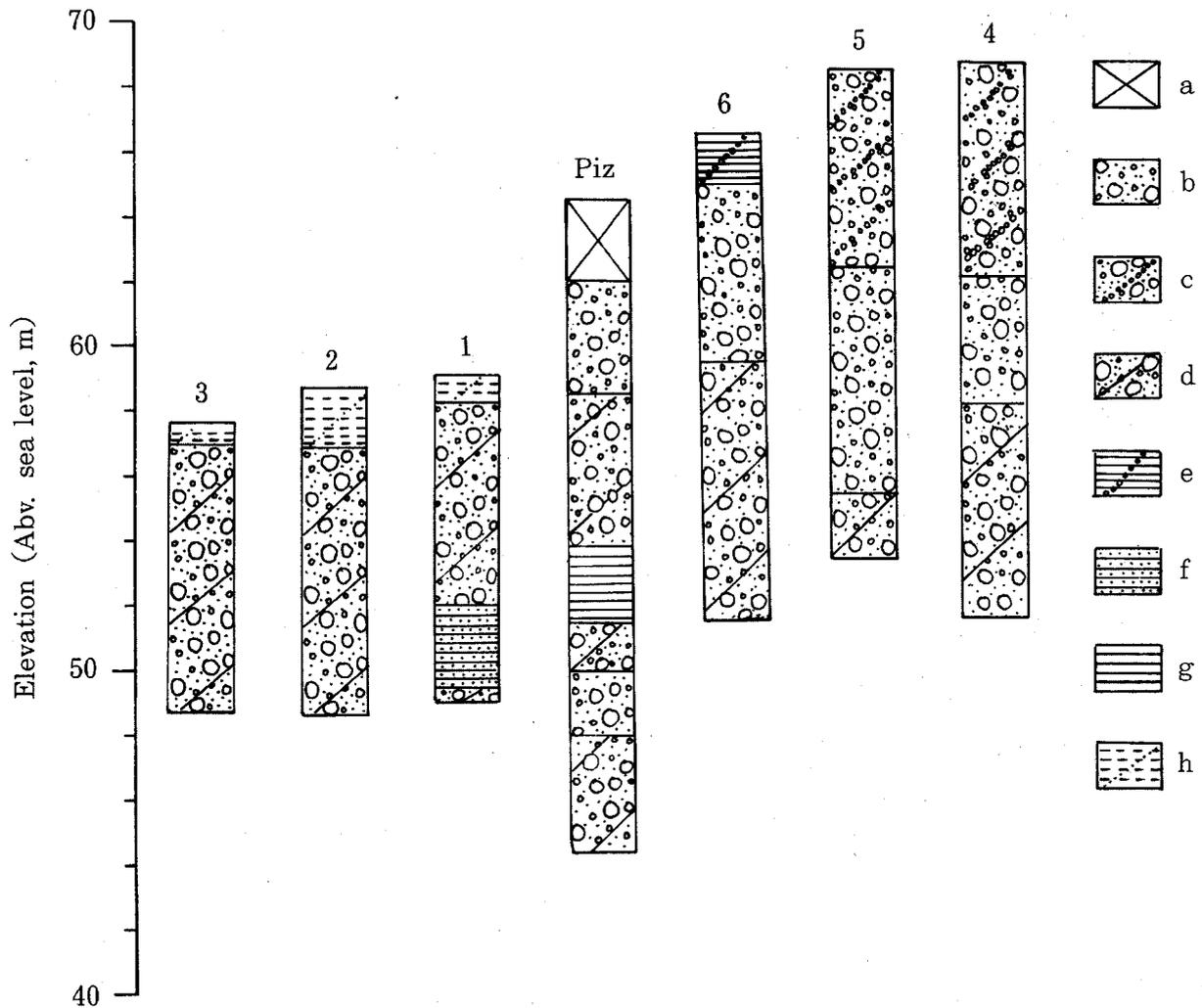
Figure 5-1. Geologic columnar section at the site of observation wells and piezometer
