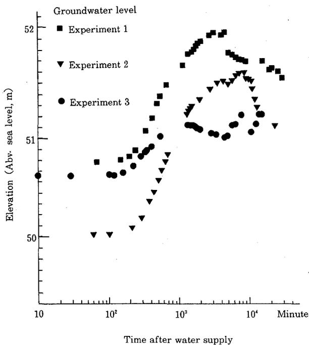
**Figure 6. Rise of the groundwater levels after supplying water to artificial recharge basin (ARB) No.1**
