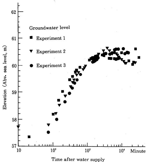
**Figure 10.** Rise of the groundwater levels after supplying water to artificial recharge basin (ARB) No.2
