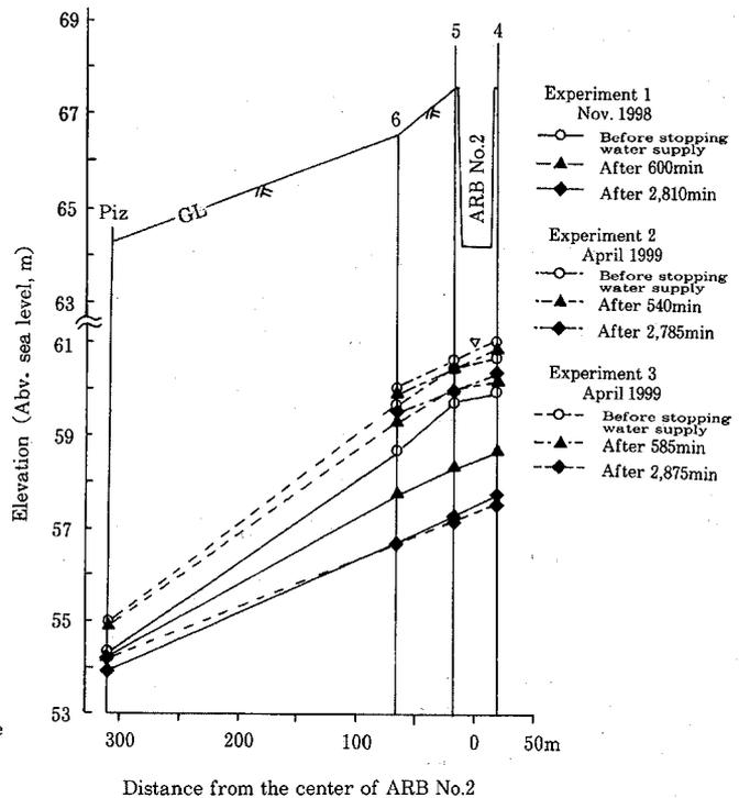
**Figure 13. Changes of longitudinal profile of the water table between observation well 4 and piezometer: after stopping water supply to artificial recharge basin No.2**
