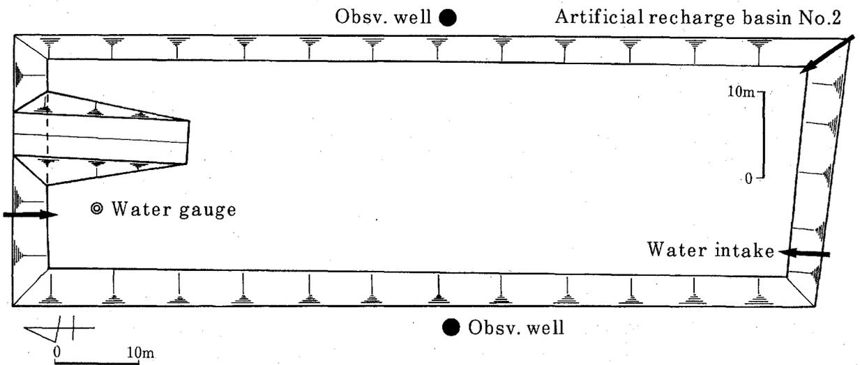
Figure 4. The form of artificial recharge basins No.1 and No.2
