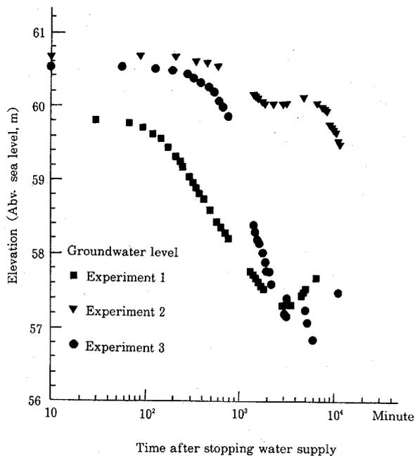
**Figure 12. Decline of the groundwater levels after stopping water supply to artificial recharge basin (ARB) No.2**
