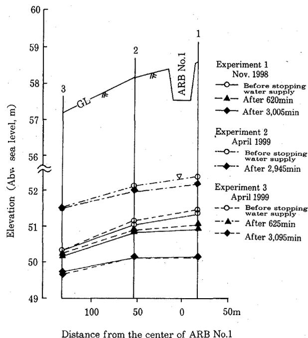
**Figure 9. Changes of longitudinal profile of the water table between observation well 1 and observation well 3: after stopping water supply to artificial recharge basin No.1**
