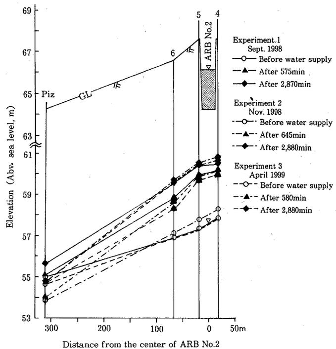
**Figure 11.** Changes of longitudinal profile of the water table between observation well 4 and piezometer: after supplying water to artificial recharge basin No.2
