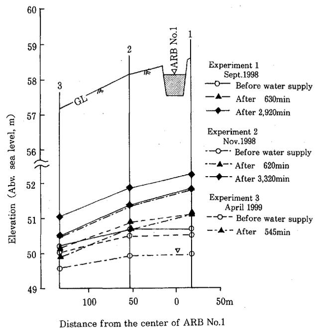
**Figure 7. Changes of longitudinal profile of the water table between observation well 1 and observation well 3: after supplying water to artificial recharge basin No.1**
