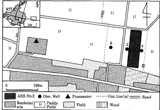
Figure 3. Artificial recharge basin No.2, observation wells 4-6, piezometer, and surround
