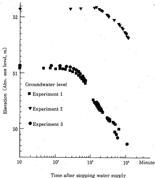
**Figure 8. Decline of the groundwater levels after stopping water supply to artificial recharge basin (ARB) No.1**
