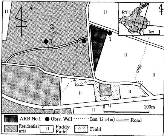
Figure 2. Artificial recharge basin No.1, observation wells 1-3, and surround
