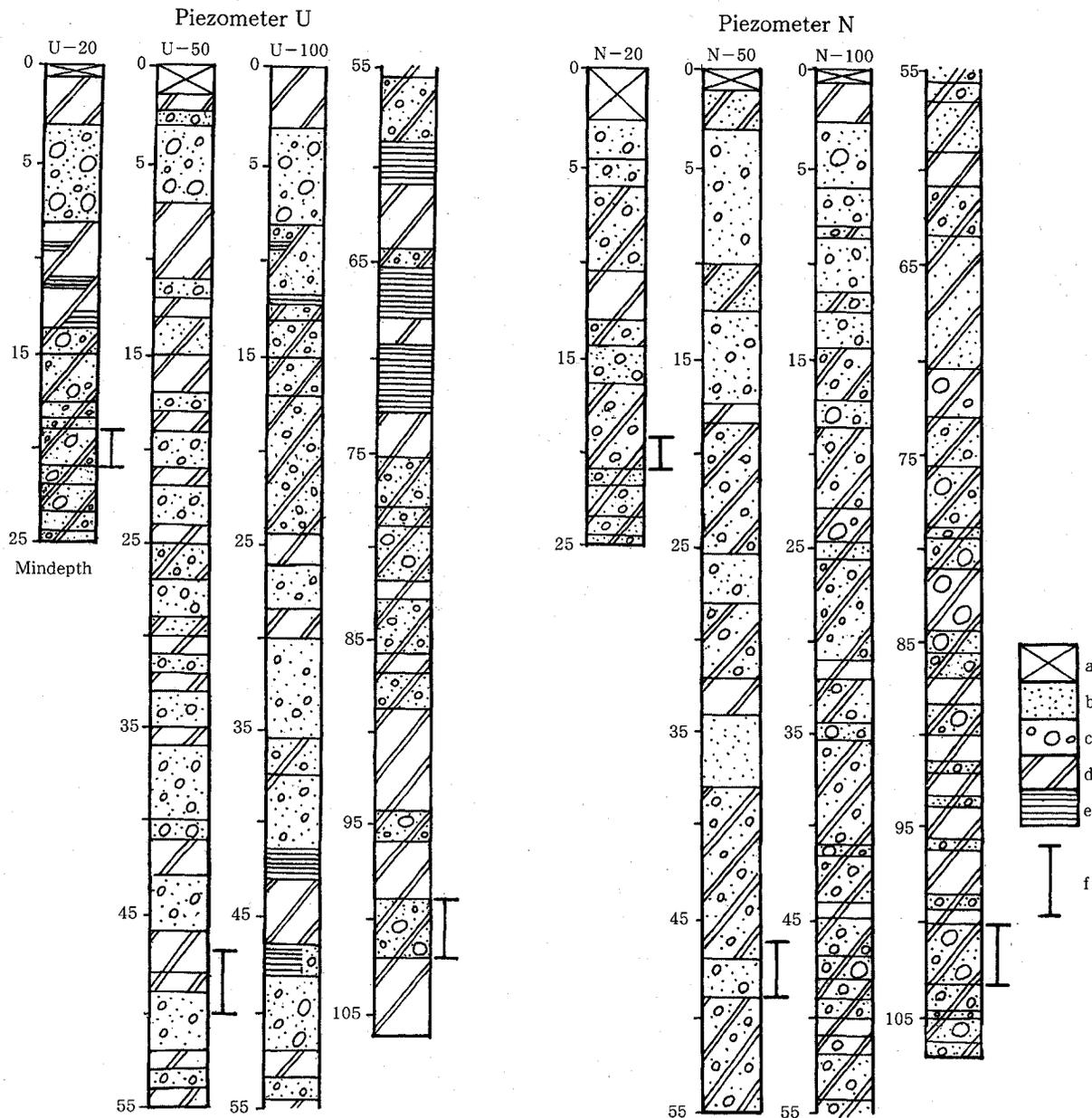
Figure 5-2. Geologic columnar section at the site of piezometers U and N
