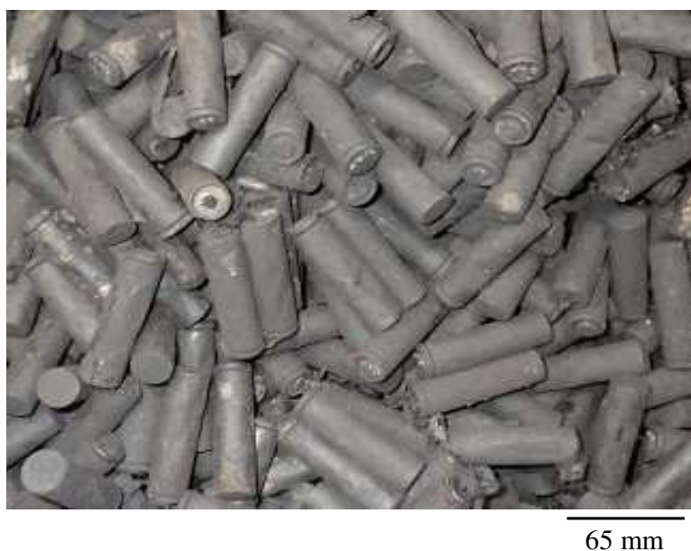
Fig. 3 Burned product (1) after LIB packs heat treatment.
