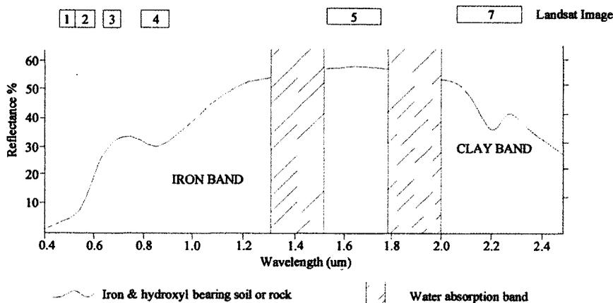
Fig. 3. A reflectance profile of the visible and IR parts of the emission spectrum, showing the changing reflectance profile of soil associated with special materials.
