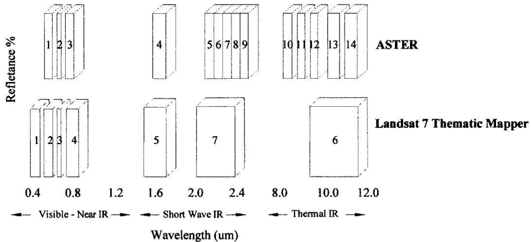
Fig. 4. Comparison of spectral bands between ASTER and Landsat7 Thematic Mapper.
