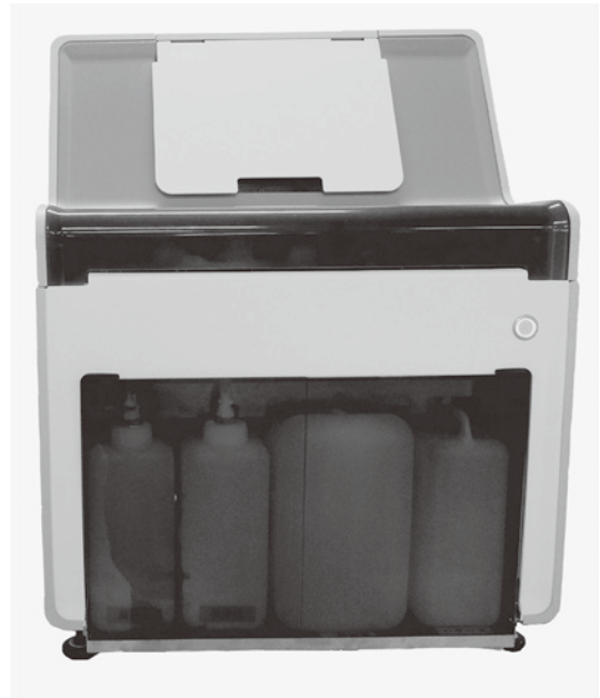
Figure 1. One-step, fully automated rapid ISH (Auto-RISH) device used to apply a high-voltage, low-frequency alternating current (AC) electric field. The new device automatically performs the denaturation and hybridization step, anti-DIG/DNP step, AP/HRP step, AP chromogenic reaction step, HRP chromogenic reaction step, and slide washing step.
