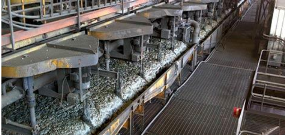
Figure 1. 13. Plant flotation circuit (Source: http://www.miningeducation.com/2016/02/flotation-cell-for-mineral-separation )
