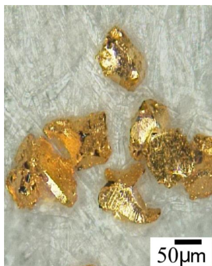
Fig. 2-13 Image of Au-coated FILCT (the thickness of gold was 100 nm).
