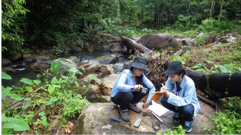
Fig. 4.1 Measurement of magnetic susceptibility of granitoids using SM30 magnetic susceptibility meter.
