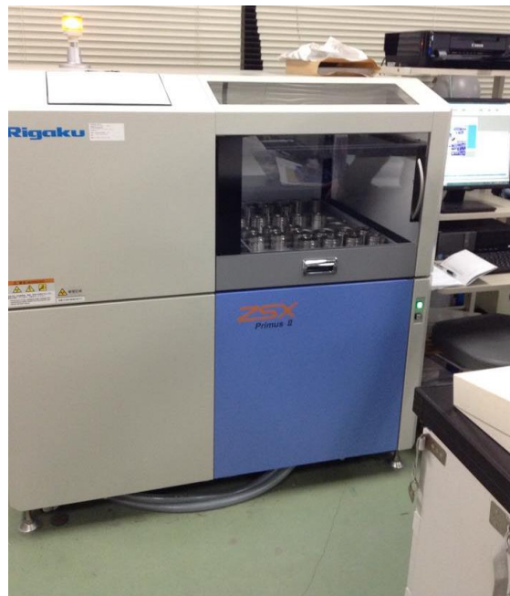
Fig. 4.12 Rigaku ZSX Primus II X-ray Fluorescence (XRF) spectrometer at Akita University
