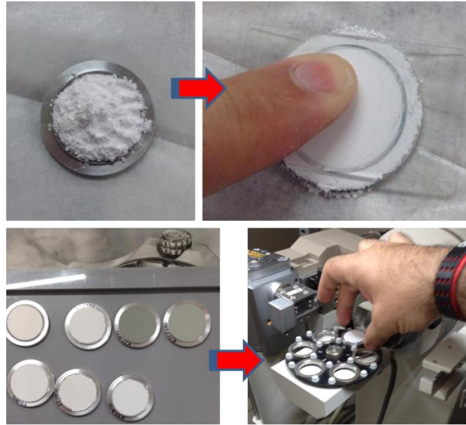
Figure 4.4 Sample preparation for XRD analyses.
