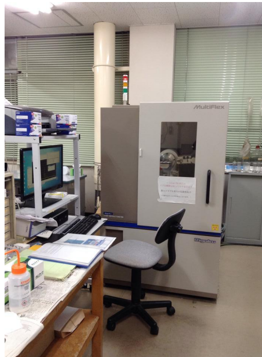
Figure 4.5 Rigaku Multi Flex X-ray Diffractometer at Department of Earth Science and Technology, Akita University.
