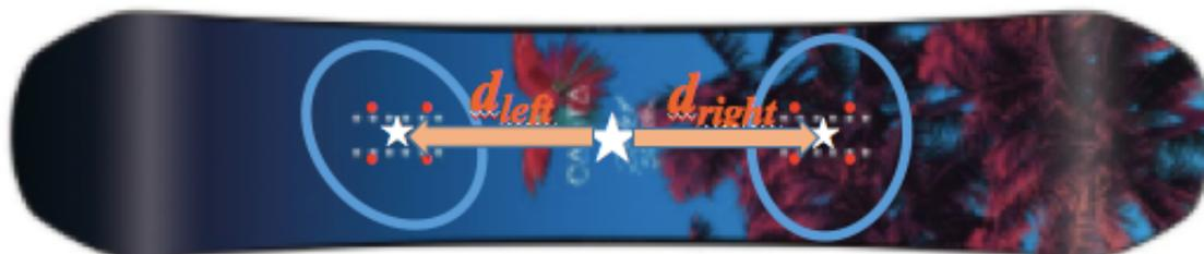
Fig.3.4 Position vectors from the original point of snowboarding to the one of the measurement systems
