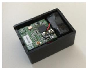
Fig. 5.1 Compact wireless motion sensor system
