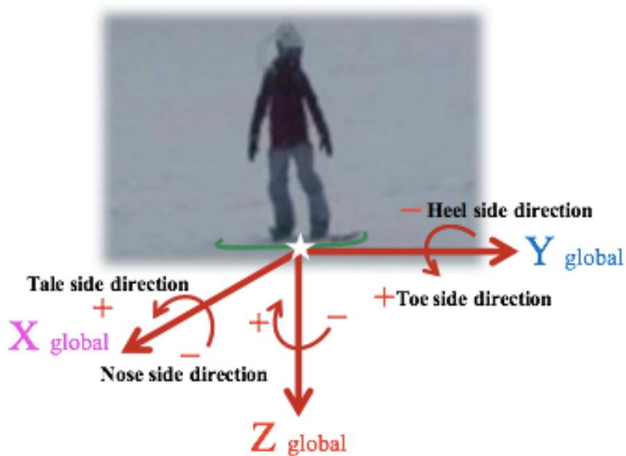
Fig.4.4 Definition of coordinate system
