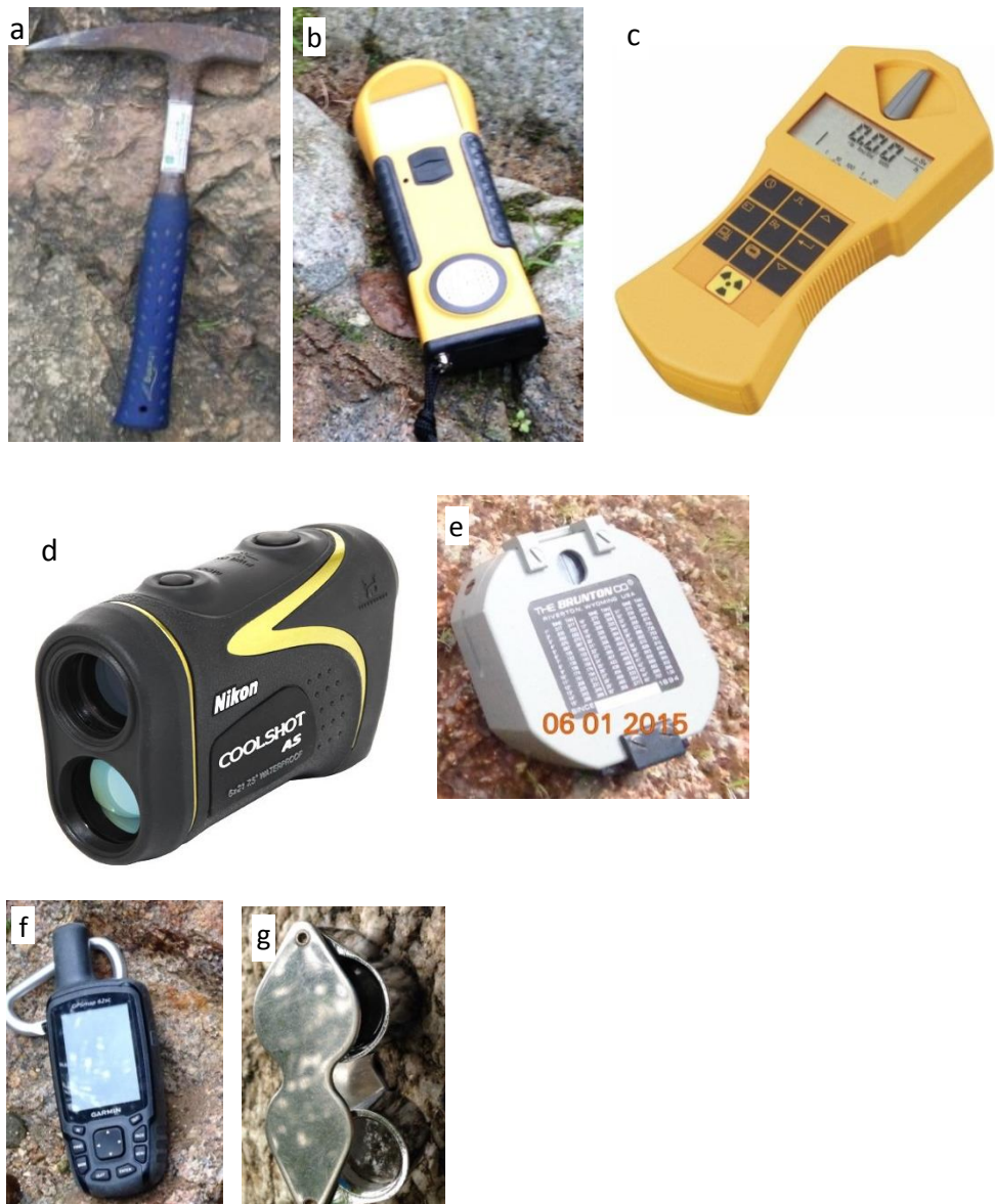
Fig. 3.1 a. hammer, b. magnetic susceptibility meter, c. gamma spectrometer, d. laser range finder, e. Brunton compass, f., g. global positioning system (GPS), and g. loupe.
