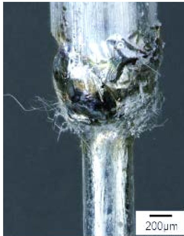
Fig.4.2.1 Whisker formation at lead wire weld.
