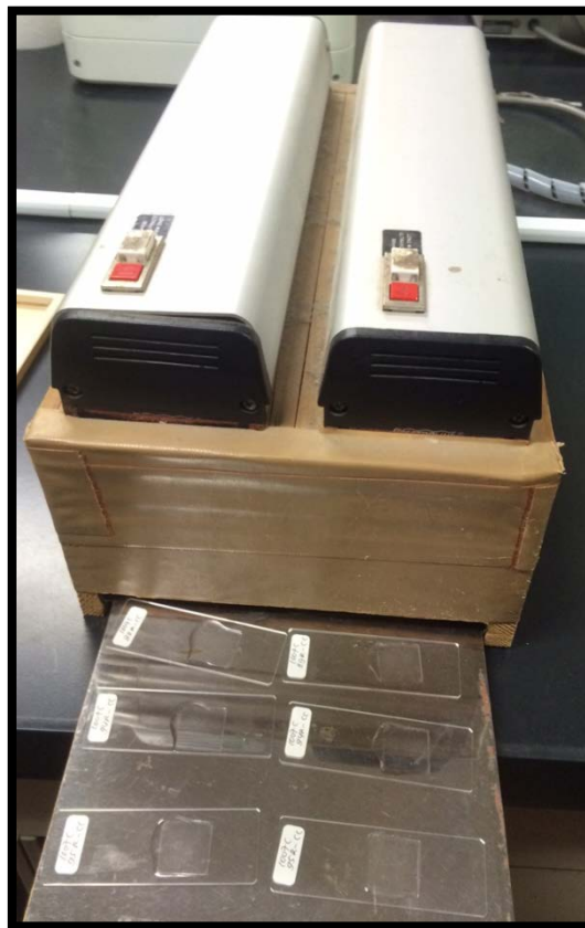
Figure 4.10. Put the cover glass under UV-curing adhesive for dry around 2 or 3 minutes.
