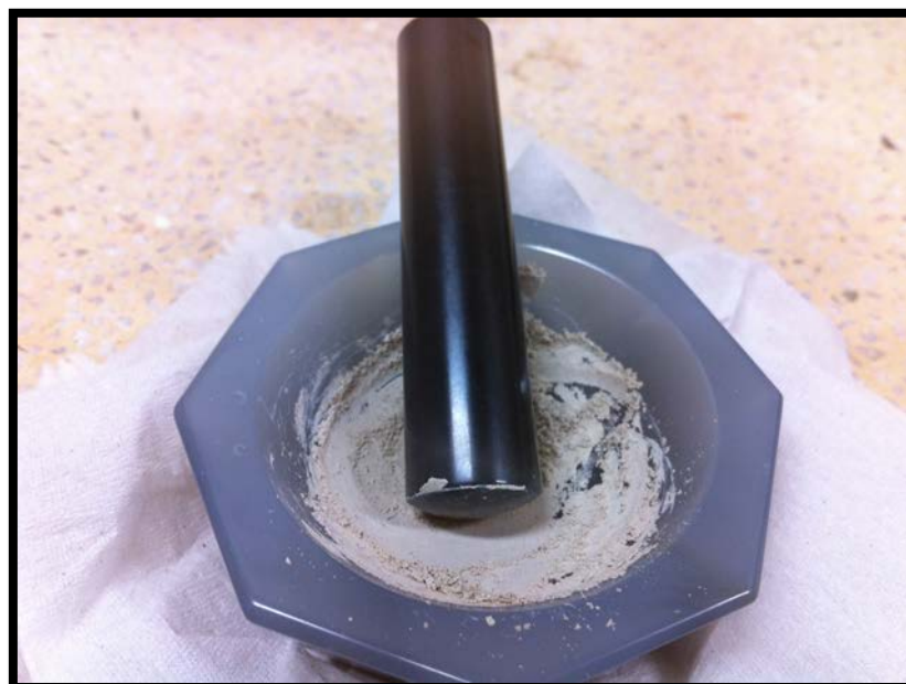
Figure 4.2. Samples were dried in an oven at a temperature around 70°C for 24 hours and powdered using a mortar.
