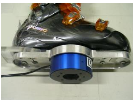
Fig.5.2 Measurement system of reaction force from snow surface
