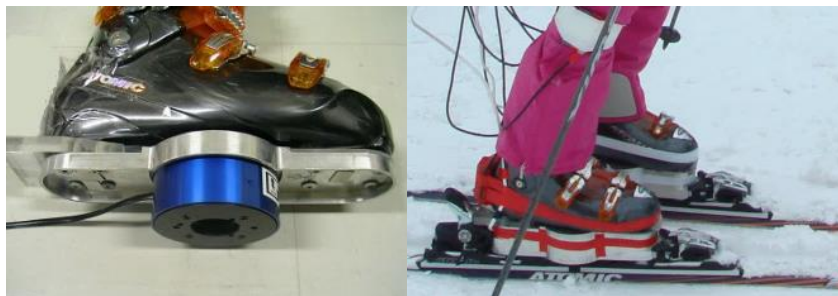
Fig.6.2 Measurement system for reaction force of snow surface
