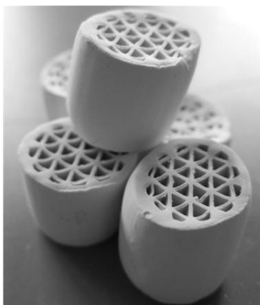
(c) Honeycomb-type 5A adsorbent
