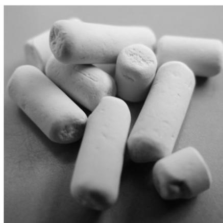
(a) Pellet-type 5A adsorbent
