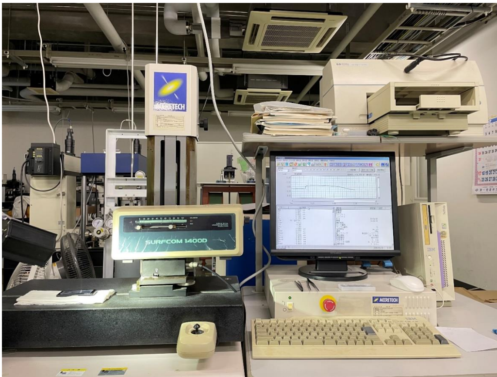
Figure 31. Image of thickness measurement instrument by using line profiles.
