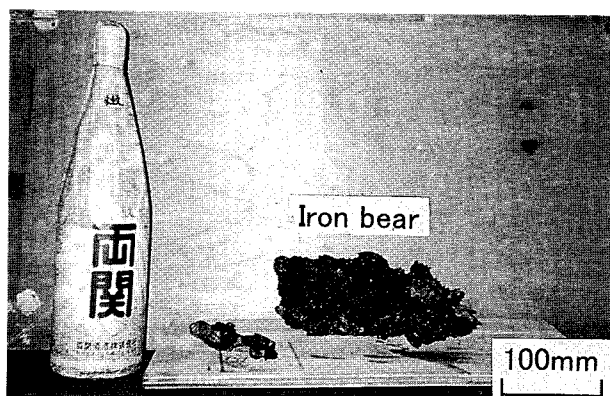
Fig. 8 Over view of the iron bear (kera) lump obtained in this experiment.
