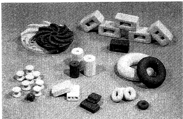
Figure 2 Various electronics parts are obtained at the same time in one powder bed by 3DP™ process. Lighter-color parts are green ceramics, while darker-color parts are sintered ceramics. They are free from the limitation of conventional methods such as dry press and sheet stack methods.
