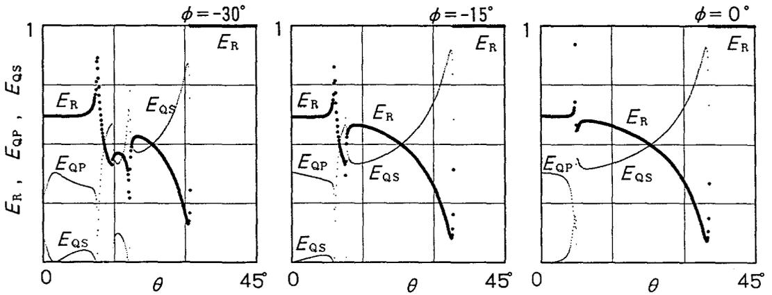
Fig. 4(a) Coefficients of power reflection,  $E_R$ , and Power transmissions,  $E_{QP}$  and  $E_{QS}$ , to the incident angle  $\theta$  for the off-angle  $\phi = -30^\circ, -15^\circ, 0^\circ$ .
