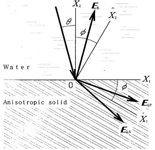
Fig. 2 Coordinates on the surface of an immersed anisotropic solid.
