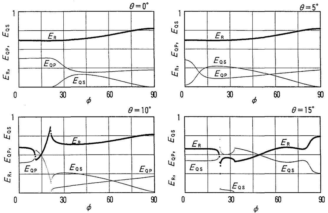
Fig. 5(a) Coefficients of power reflection,  $E_R$ , and Power transmissions,  $E_{QP}$  and  $E_{QS}$ , to the off-angle  $\phi$  for the incident angle  $\theta = 0^\circ, 5^\circ, 10^\circ,$  and  $15^\circ$ .
