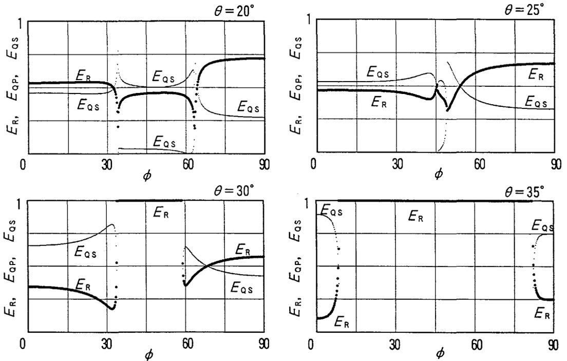
Fig. 5(b) Coefficients of power reflection,  $E_R$ , and Power transmissions,  $E_{QP}$  and  $E_{QS}$ , to the off-angle  $\phi$  for the incident angle  $\theta = 20^\circ, 25^\circ, 30^\circ,$  and  $35^\circ$ .
