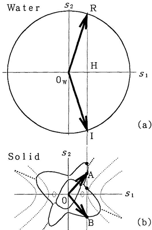
Fig. 3 Solwness curve for water (upper) and an anisotropic solid (lower).
