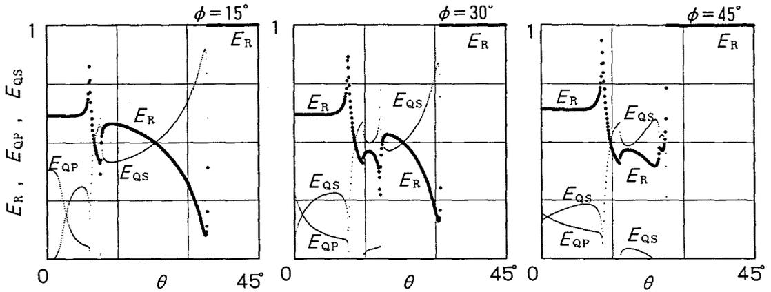
Fig. 4(b) Coefficients of power reflection,  $E_R$ , and Power transmissions,  $E_{QP}$  and  $E_{QS}$ , to the incident angle  $\theta$  for the off-angle  $\phi = 15^\circ, 30^\circ, 45^\circ$ .
