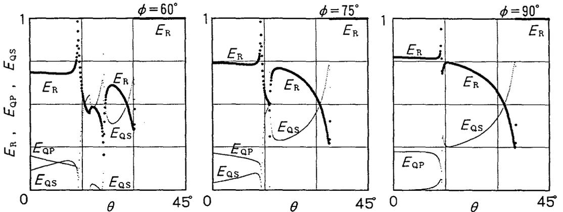
Fig. 4(c) Coefficients of Power reflection,  $E_R$ , and Power transmissions,  $E_{QP}$  and  $E_{QS}$ , to the incident angle  $\theta$  for the off-angle  $\phi = 60^\circ, 75^\circ, 90^\circ$ .
