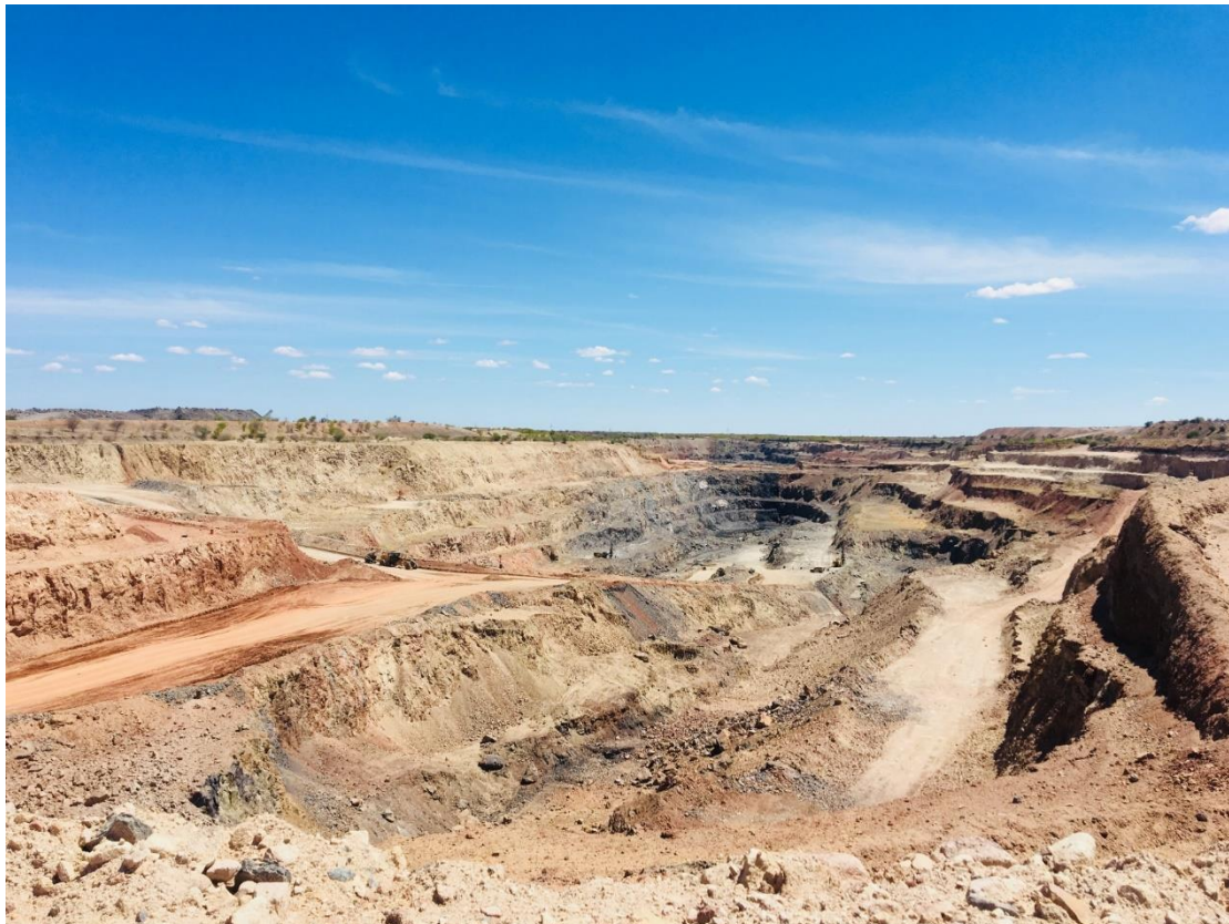
Figure 8: A photo showing a section of the mining pit. The mining follows the Bushman Lineament indicated by the black graphitic schists where the veins and breccias occur.
