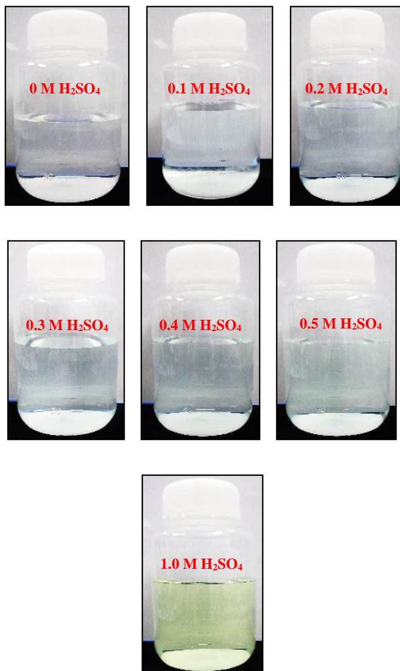
Fig. 2.11 Pregnant leach solutions obtained after high-pressure oxidative leaching under the condition of 0, 0.1, 0.2, 0.3, 0.4, 0.5, and 1.0 M.
