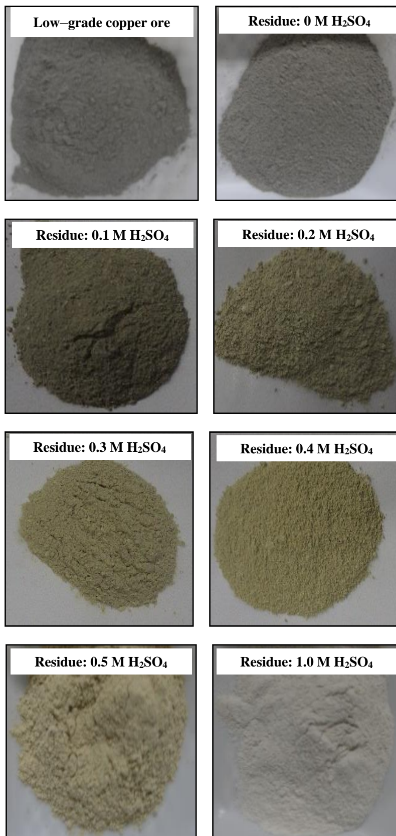
Fig. 2.12 Photograph of the low-grade copper ore and residues obtained after high-pressure oxidative leaching under the condition of 0, 0.1, 0.2, 0.3, 0.4, 0.5, and 1.0 M.
